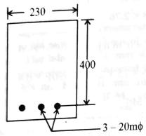
$\sigma cbc = 7 \text{ N/mm}^2$  $\sigma st = 230 \text{ N/mm}^2$
