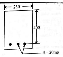
$\sigma cbc = 7 \text{ N/mm}^2$  $\sigma st = 230 \text{ N/mm}^2$
