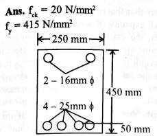
Force of tension =  $0.87\sigma_{v}$  Ast  $= 0.87 \times 415 \times 4 \times 490 = 708 \text{ kN}.$
